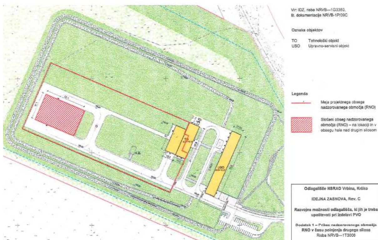
Figure 113: The boundaries of the controlled area at the repository with two silos present. Source: IBE d.d., Development potentials of the repository to be taken into account in elaboration of the EIA, Addendum 1 – Outline of the controlled area (CRA) during the filling of the second silo, Drawing NRVB---1T3006.
