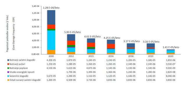
*Figure 3: The history of core damage frequency due to internal initiating events, external initiating events from the power plant and external initiating events from the surroundings*
