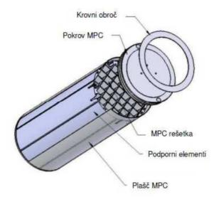
Figure 5: Spent fuel multi-purpose canister (MPC)
