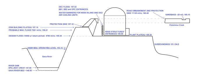
Figure 2: Flood protection
