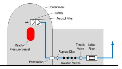
Figure 4: Schematic diagram of passive containment filtering vent system
