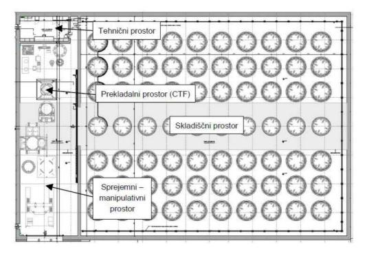
Figure 6: Floor plan of SF dry storage building
