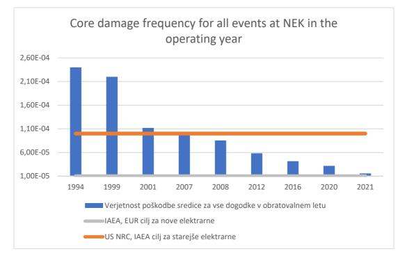
Figure 7: Safety level measured with core damage frequency per operating year (CDF/yr)
